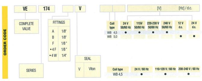
Note: Valve supplied with coil in a multipack.
